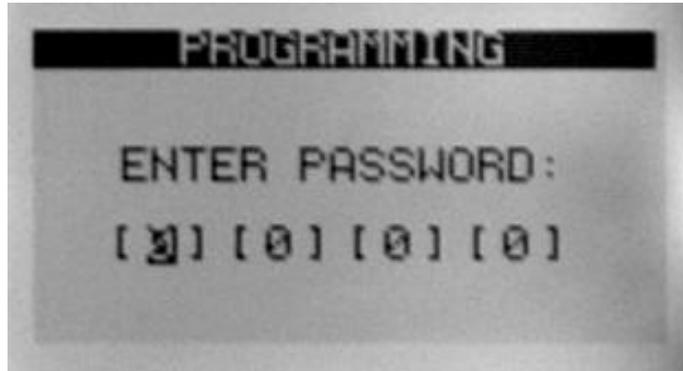
A 4 digit password must be entered using **ACK/RESET**, ▼ and ► buttons.
